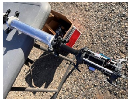
The lead segment of a pipe crawler is equipped with a camera, mock-up radiation scanner and other sensors. A 3D printer was used to help build the crawler.
