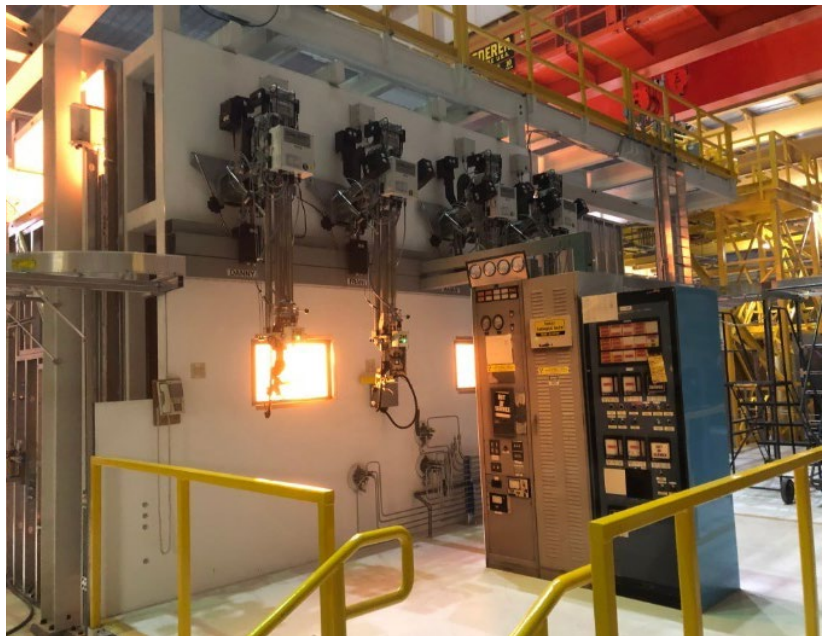
Workers recently installed manipulator equipment at a full-scale mock-up of areas of the Hanford Site's Waste Encapsulation and Storage Facility that will be used to move nearly 2,000 radioactive capsules from underwater storage, into steel and concrete casks and loaded onto a truck for a short trip to a secured storage area near the facility.
