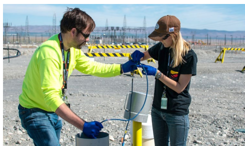
A remote sensor developed by Freestone Environmental Services of Richland is helping track the movement of the chromium underground.
