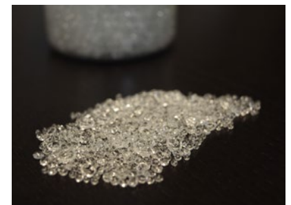
Glass beads, called frit, are added to the melter in the Low-Activity Waste Facility, where it melts at 2,100 degrees Fahrenheit. Local business Fluid Controls and Components Inc. supplied the frit.
