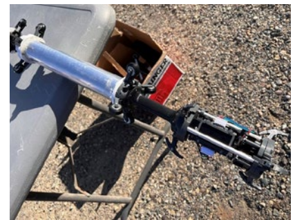
The lead segment of a pipe crawler is equipped with a camera, mock-up radiation scanner and other sensors. A 3D printer was used to help build the crawler.
