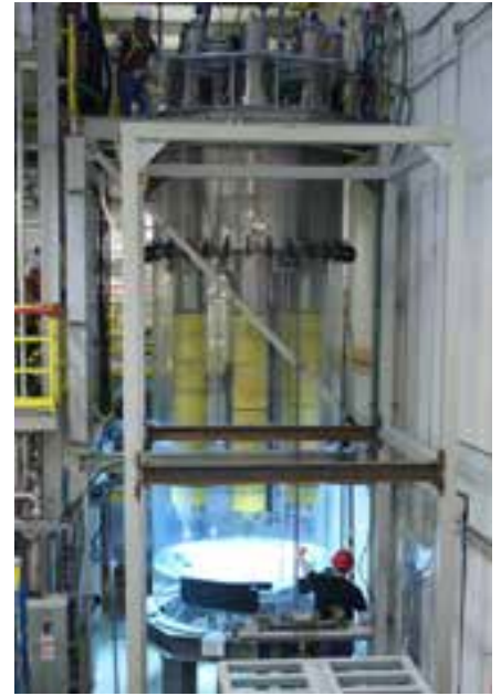
Workers used a clear plastic vessel for half-scale testing of the WTP pulse-jet mixer/vessel mixing system.
