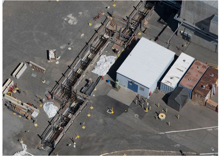
This aerial photo shows trenches dug for the replacement of approximately 1,300 feet of piping between the 242-A Evaporator and an adjacent tank waste storage area near the center of the Hanford Site.
